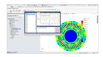
2D Simplification: Automatically extracts a 2D model from a 3D model Make the geometrical transition effortless and fast, especially for complicated models
