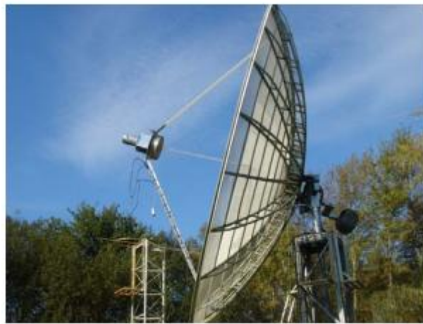
Figure 1 :The feed with parabolic reflector used for sun noise measurement
