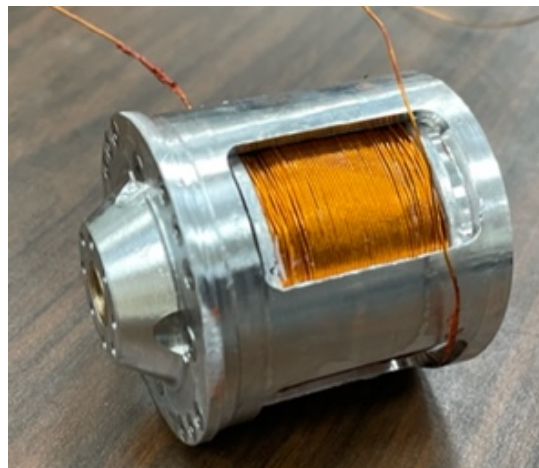
Fig. 4: Actual coil used for the proposed spring
