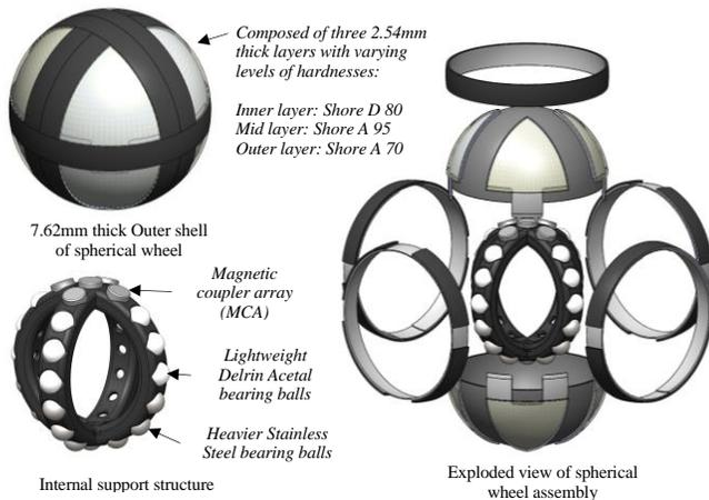
Figure 11: Design of spherical wheel for MCBD proof-of-concept prototype
