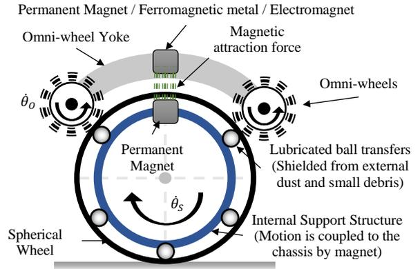
Figure 2: 2D schematic of magnetically coupled ball drive (MCBD) concept
