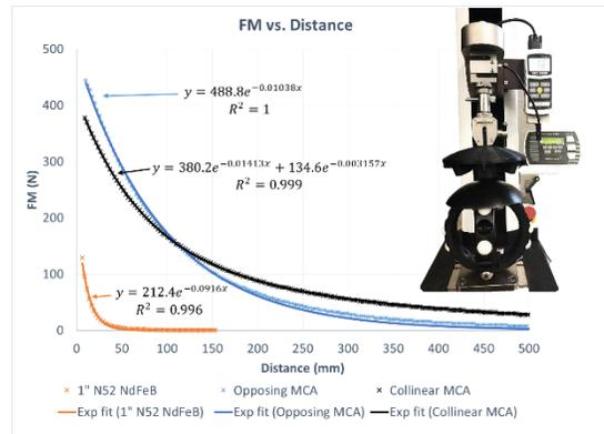
Figure 10: Experimental verification of simulation results using motorized force test stand
