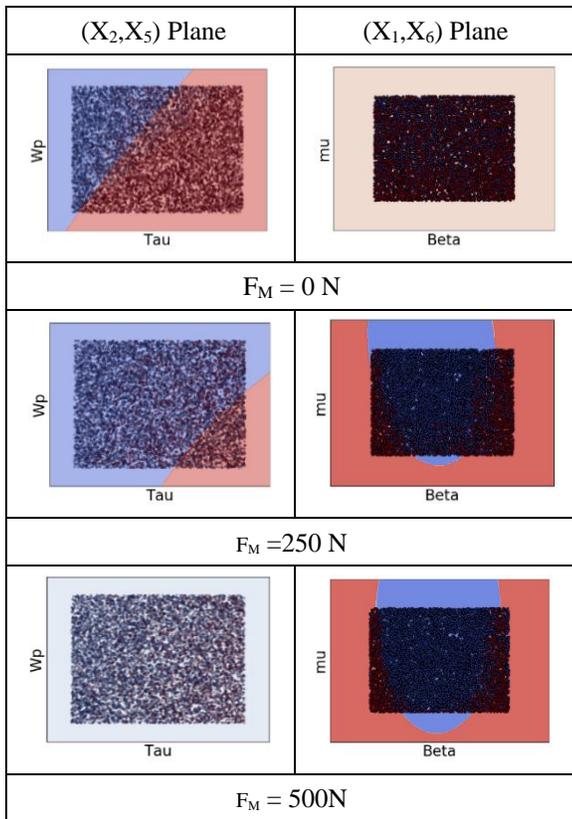
Figure 5: Slip (red) and No-Slip (Blue) surfaces based on two feature classification with 10,000 training samples.
