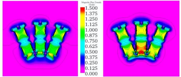
Figure 9: Magnetic flux density for the collinear and opposing MCA designs. Significant increase in magnetic flux density is achieved using the opposing MCA design. Extent of magnetic field is also more contained using opposing MCA design.
