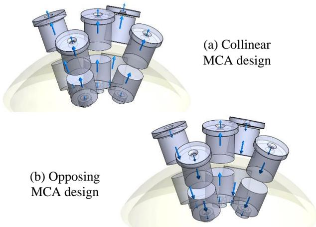
Figure 8: Magnetic Coupler array (MCA) designs evaluated for MCBD concept
