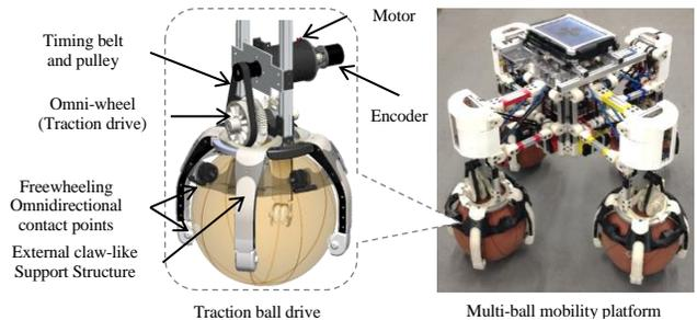
Figure 1. Example of traction ball drive used in authors' prior work [4] for a holonomic multi-ball mobility platform
