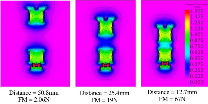
Figure 7: Magnetic flux density and corresponding  $F_M$  values for a pair of 25.4mm x 25.4mm cylindrical N52 NdFeB magnets at three coupling distances.
