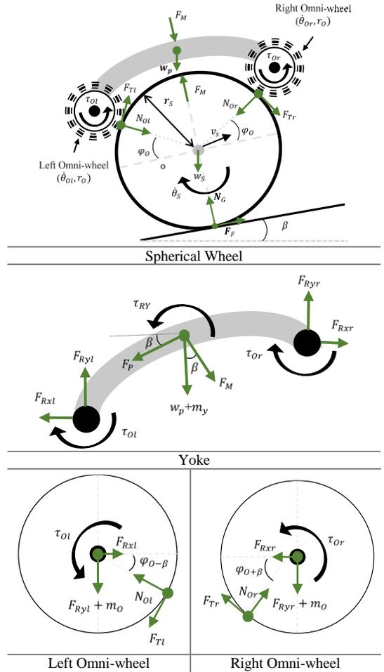
Figure 3: Free body diagram for simplified 2D model of magnetically coupled ball drive
