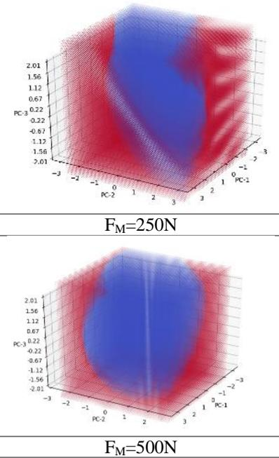
Figure 6: Feasible design space (blue) shown with respect to three principal components. The increase in  $F_M$  from 250N to 500N is shown to increase the feasible space by 35%.
