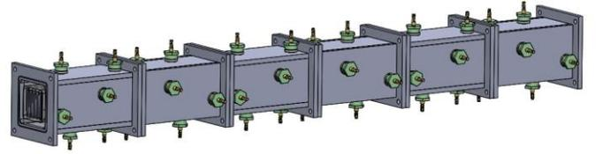
Figure 5. Ohmic-heater assembly
