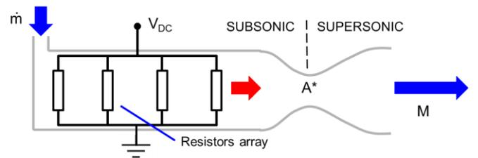
Figure 1. Schematic of an ohmic-heater for a high-enthalpy hypersonic wind tunnel.
