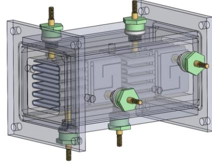
Figure 4. Resistor array module
