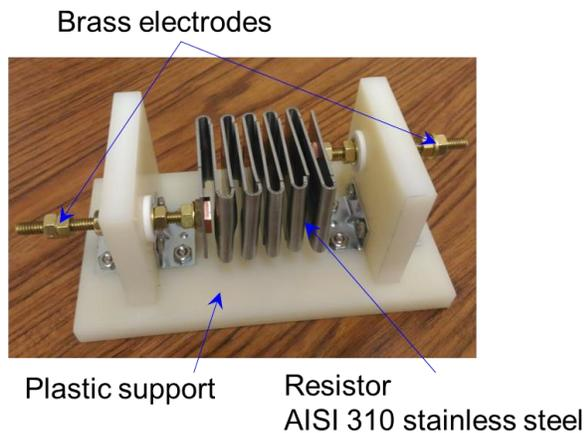
Figure 10. Prototype of the design 1 resistor for preliminary testing.
