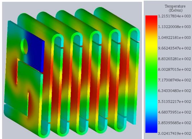
Figure 6. Design 1 temperature profile after 15 s.
