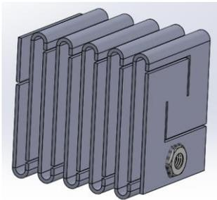
Figure 2. Individual resistor. The electrodes thread into the nuts, which are fastened onto the resistor
