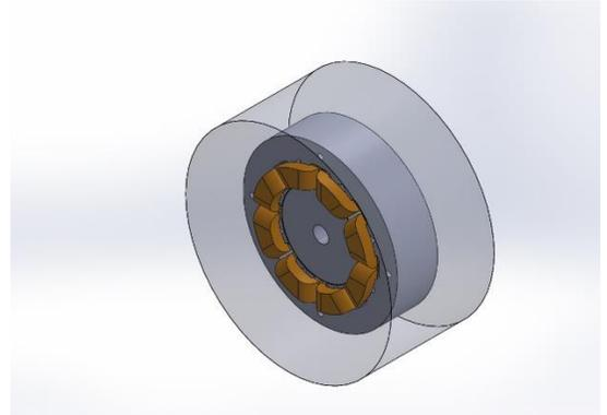
Figure 1. Solidworks model of the Active Magnetic Bearing
