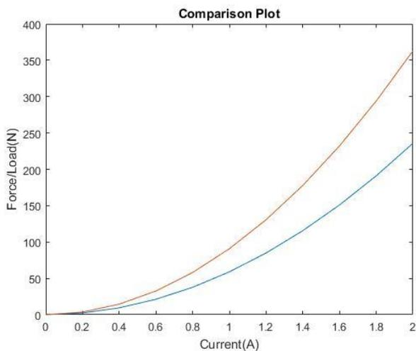
Figure 9.2 Comparison plot of the results (red line denotes Simulation results and blue line denotes the experimental results)
