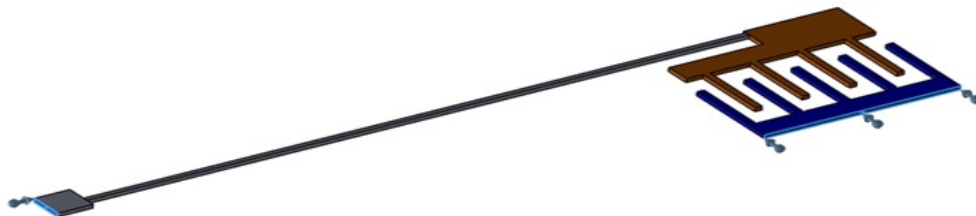
Figure 4 - Fixed constraint applied on the fingers
